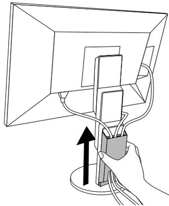
2. While holding down
