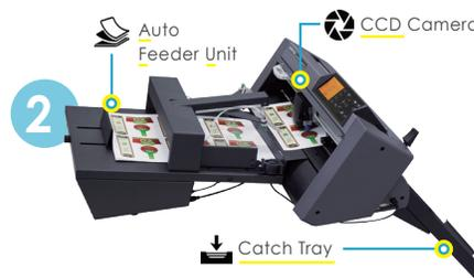
Loaded sheets are automatically placed into the Graphtec machine to contour / perforation cut.
