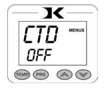
this odometer instead. The arrow keys no longer adjust the countdown timer, but instead are used to set the countdown odometer. When OFF, the timers are visible.
