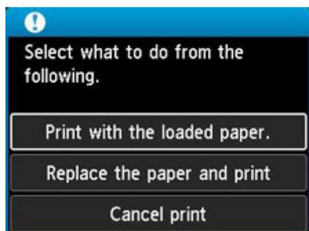
Select the appropriate action using the ▲▼ buttons and press the printer's **OK** button.
