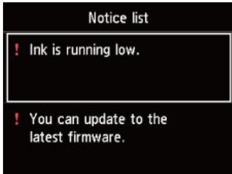
Use the ▲ ▼ button to select a message and press the **OK** button to view the message details screen to check the details and take action.
