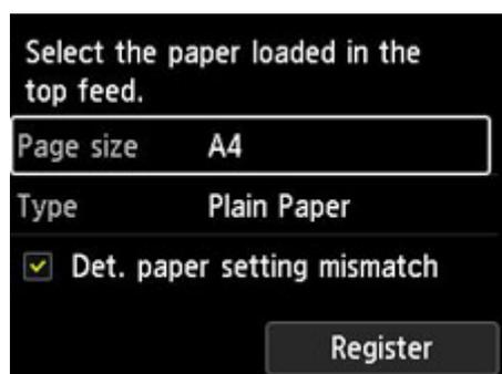
If the loaded paper matches the paper information displayed on the printer's LCD, select **Register** using the ▲▼ buttons and press the printer's **OK** button.
