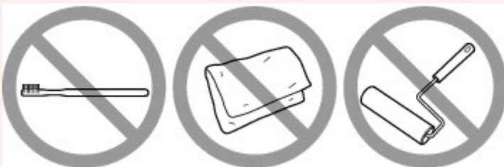
Not OK - brush made from hard material, cloth or washcloth, sticky and abrasive materials.
