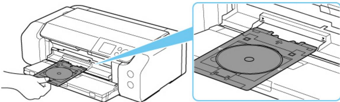
6. Insert multi-purpose tray straight in in horizontal direction until arrow (▼) on multi-purpose tray guide is approximately aligned with arrow (▲) on multi-purpose tray.
