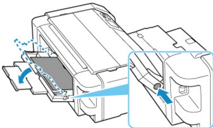
2. Slowly pull out paper, either from paper output slot or from manual feed tray, whichever is easier.
