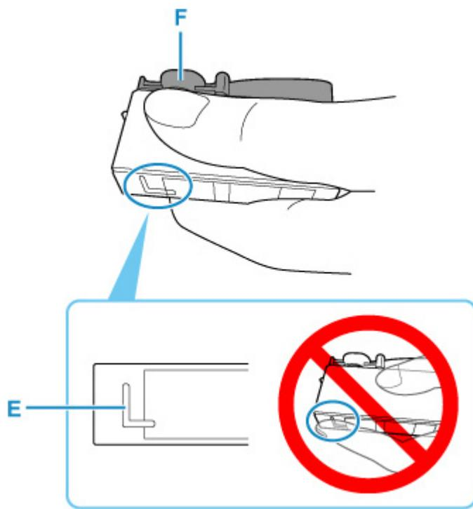
6. Twist the orange protective cap (F) 90 degrees horizontally to remove it off GENTLY.
