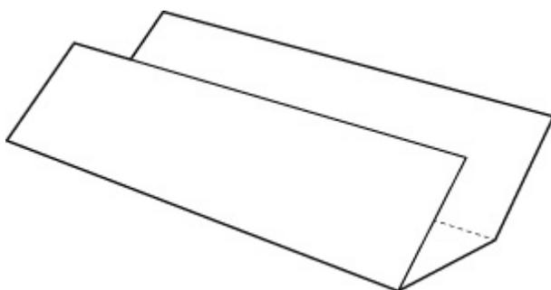
7. Load this sheet of paper sideways in the top feed with the open side facing you.
