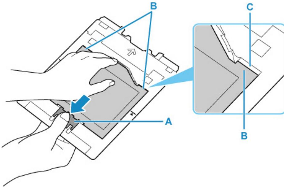
4. Peel a sheet of Printable Nail Stickers from adapter.
